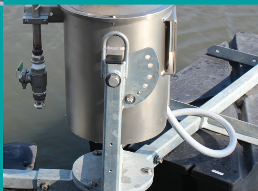
Indexable head for fan inclination of 0-90 degrees
