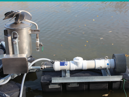
Pump holder for ease of pump inspection and maintenance
