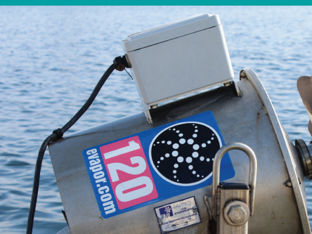
Optional vibration switch to automatically shutdown the fan from scale build-up on the propeller and protect from premature motor failure from fan imbalance. Comes housed in a second enclosure to provide additional protection against water ingress.
