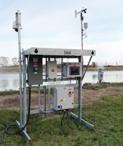
Single unit 420F (floating) Evaporator system with premium automation package
